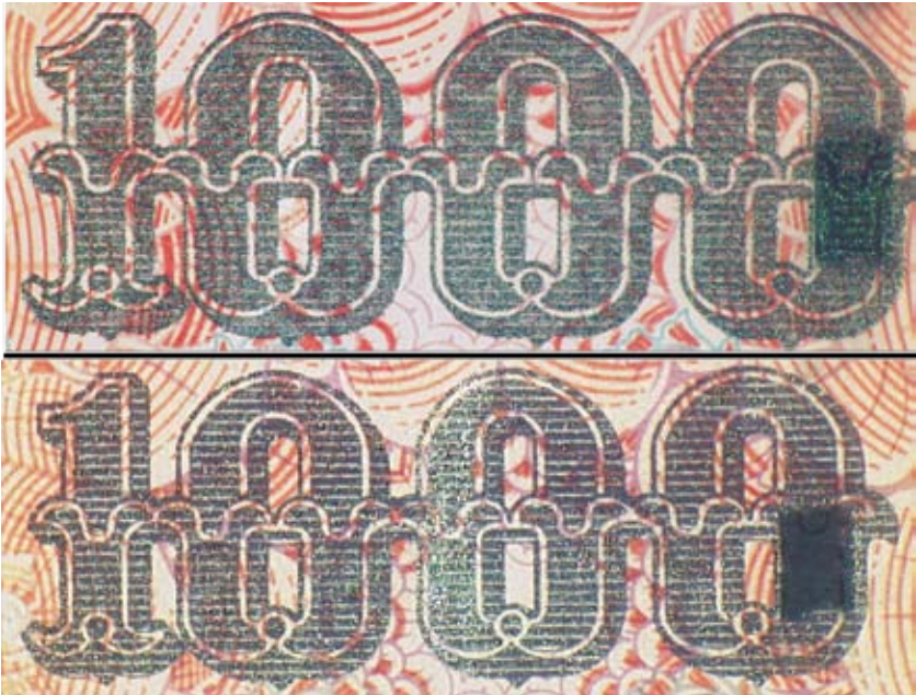
Figure 5: Optical Variable Ink of Genuine (upper) & Counterfeit (lower) Currency
