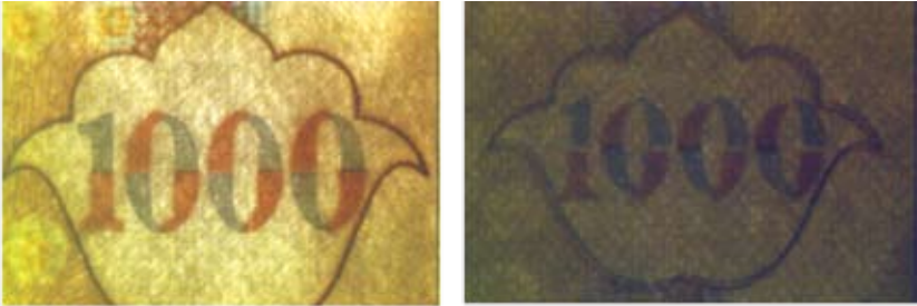
Figure 4: See-through Register of Genuine (left) & Counterfeit (right) Currency
